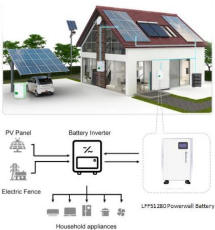
Figure 2. ST-51280F standard battery application scenario
