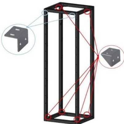
Step3. Lock the screws of 8 small triangles (6 at the bottom of the shelf and 2 at the back of the top)
