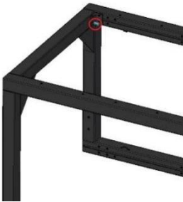
Step3. Lock the screws of 8 small triangles (6 at the bottom of the shelf and 2 at the back of the top)
